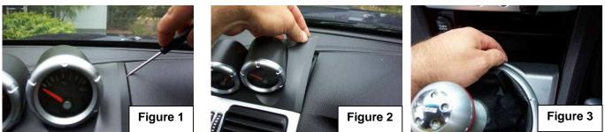
**3.**Using your hand pull up from the front the panel around the gear lever to remove. (Refer figure 3) If an automatic gear shift surround place in a suitable location.
