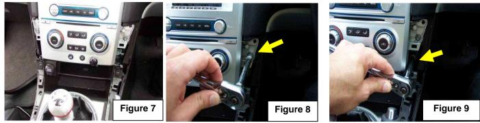
7. With a socket (8 mm) remove the 4x screws from side of ICC. 2x screws on each side. Figure 8 & 9.
